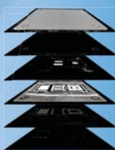
X-scan, layers inside of IC
